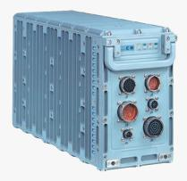
The removable front panel and top and bottom covers simplify maintenance of circuit cards, power supply and backplane I/O wiring.
