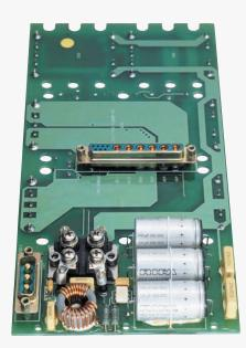
All power supplies are full military class and incorporate new generation DC/DC converters with up to 90% efficiency. Nominal input voltages are 115 VAC and 28 VDC according to MIL-STD-704.
