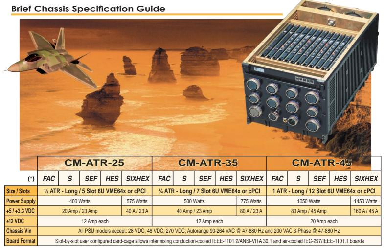
(\*) Cooling Options: FAC - Flowthrough Air Cooled; S - Sealed; SEF - Sealed, Extended Fins; HES - Sealed, Heat Exchanger Sidewalls; SIXHES - Sealed, Six Heat Exchangers
