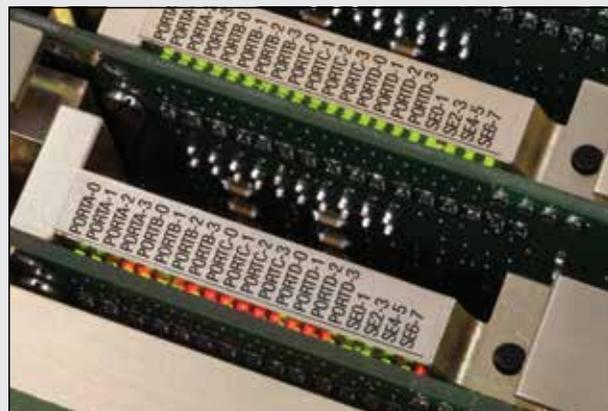
System wiring errors are detected in one slot (provoked when a front panel loop-back test connector is removed).
