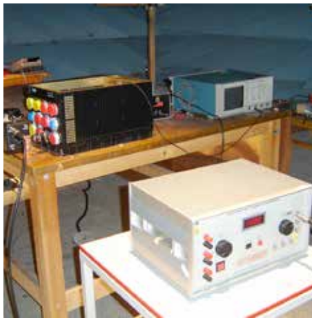
THE CM-ATR-45 PASSES ELECTROMAGNETIC IMMUNITY TEST. CONDUCTED SUSCEPTIBILITY DAMPED SINUSOIDAL TRANSIENTS, CABLES AND POWER LEADS 10 KHz to 100 MHz. MIL-STD-461E CERTIFICATE AVAILABLE.
