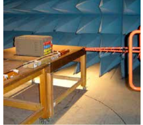
THE CM-ATR-45 PASSES ELECTROMAGNETIC EMISSION & RADIATION TEST. RADIATED E FIELD 30 MHz to 1 GHz HORIZONTAL POLARIZATION. MIL-STD-461E CERTIFICATE AVAILABLE.
