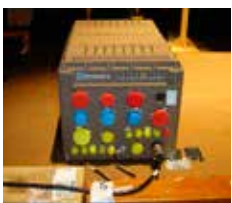
THE CM-ATR-45 PASSES ELECTROMAGNETIC EMISSION & RADIATION TEST. RADIATED E FIELD 30 MHz to 1 GHz VERTICAL POLARIZATION. MIL-STD-461E CERTIFICATE AVAILABLE.
