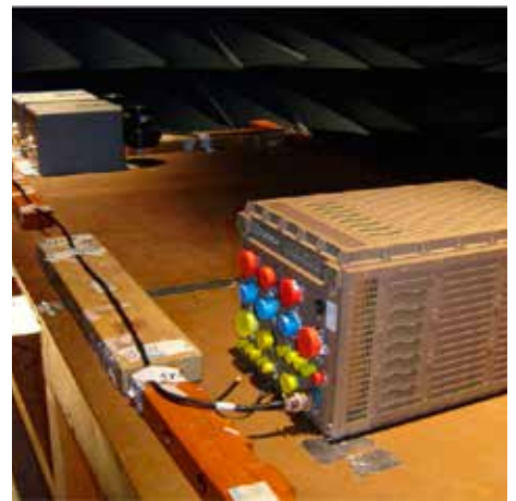
THE CM-ATR-45 PASSES ELECTROMAGNETIC IMMUNITY TEST. CONDUCTED SUSCEPTIBILITY DAMPED SINUSOIDAL TRANSIENTS, CABLES AND POWER LEADS 10 KHz to 100 MHz. MIL-STD-461E CERTIFICATE AVAILABLE.
