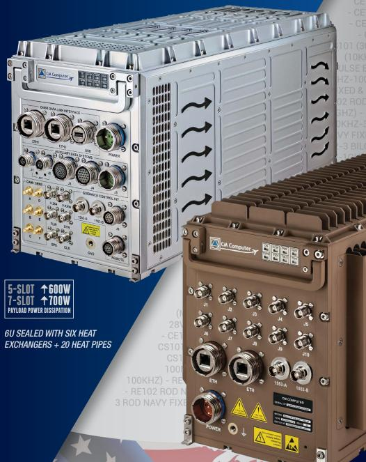
3U UP TO 150W 6U UP TO 1300W PAYLOAD POWER DISSIPATION
