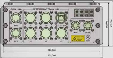
The MIL COTS Switch is mounted as standard via six M4 bottom cover threads that provide secure attachment to the application vehicle base plate. Other mounting options are available upon request. These include side or rear panel fixings, protruding bottom cover legs, front NAS-622 hooks and self-clinching pilot pins, or other.
