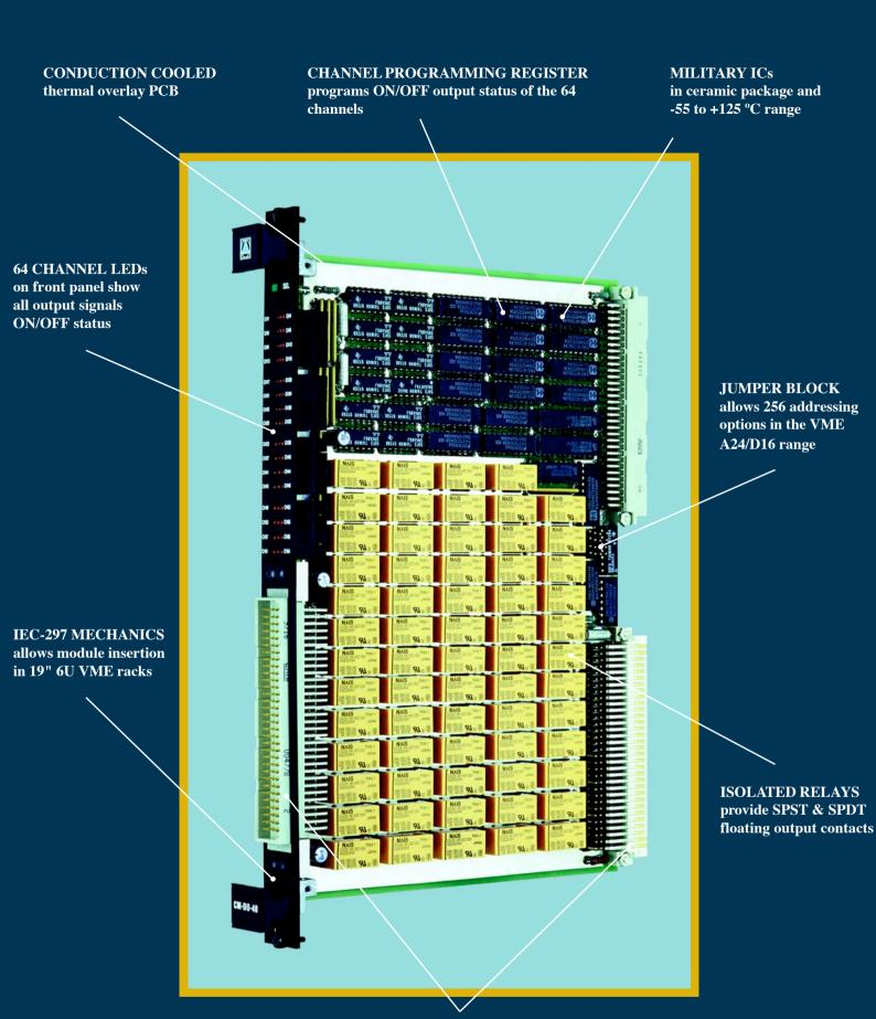
CLASS I MIL C-55302 & MIL C-24308 CONNECTORS withstand > 500 insertion cycles
