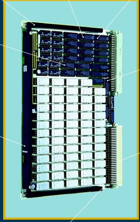
THERMAL PASTE behind ICs improves heat dissipation with the thermal overlay
