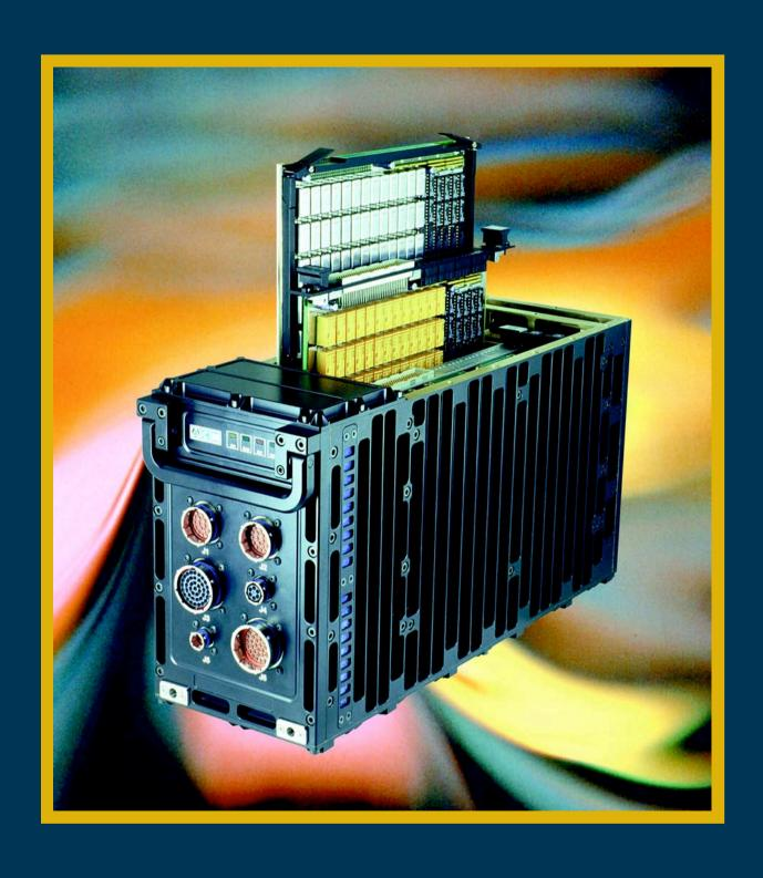
CM-DO-40 Modules inserted in CM-RA-20/AV ATR Avionics Enclosure
