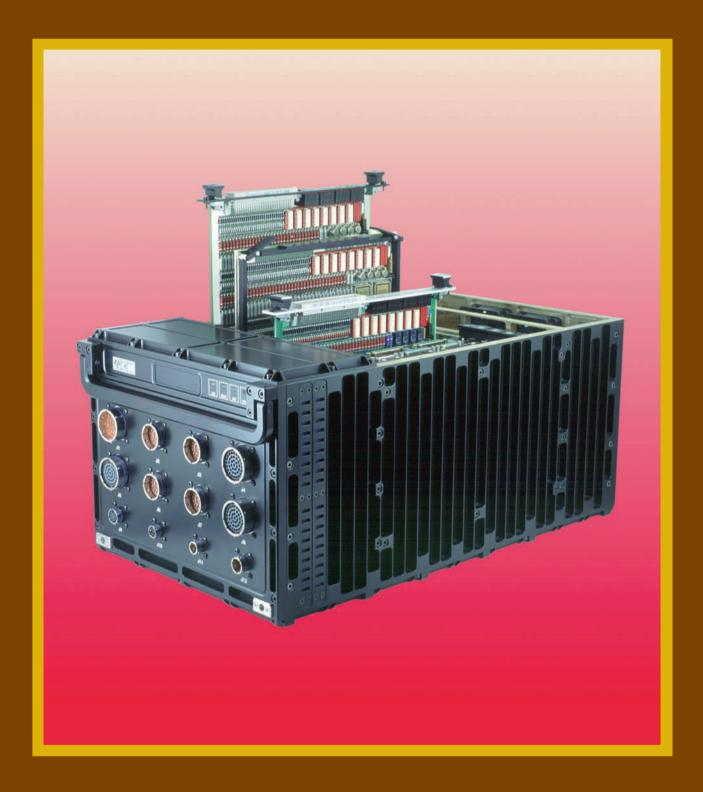
CM-DI-40 Modules inserted in CM-RA-40/AV ATR Avionics Enclosure
