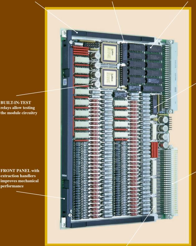
THERMAL PASTE behind ICs improves heat dissipation with the thermal overlay
