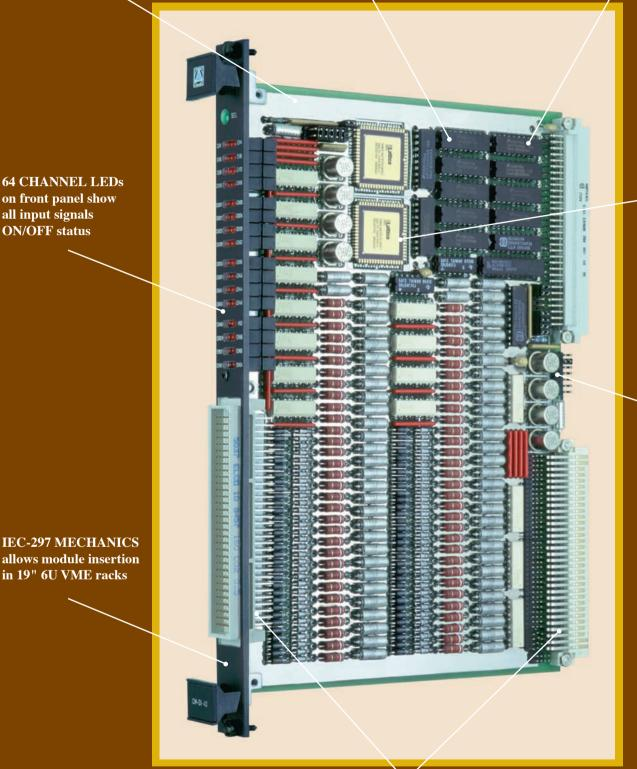
**VME INTERRUPTER** offers programable level and supplies a unique **ID-vector for each group** of 16 input channels
