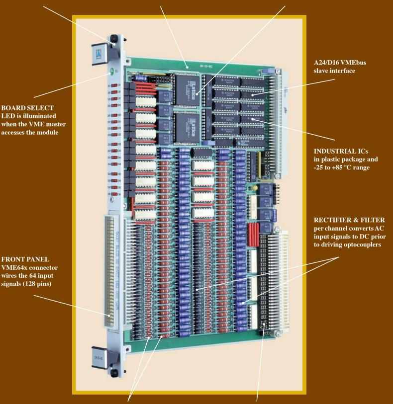
INPUT PROTECTION Resistor and Zener prevents channel overvoltage damage JUMPER BLOCK wire-removes all input signals from P2
