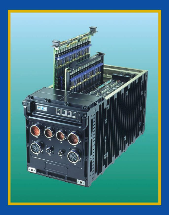
CM-DA-40 Modules inserted in CM-RA-30/AV ATR Avionics Enclosure
