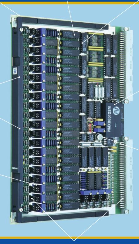
JUMPER BLOCK allows 256 addressing options in the VMEbus A24 range
