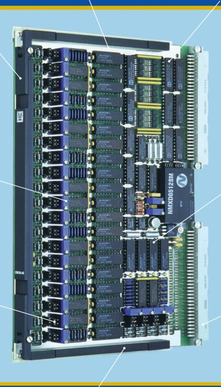
THERMAL PASTE behind ICs improves heat dissipation with the thermal overlay
