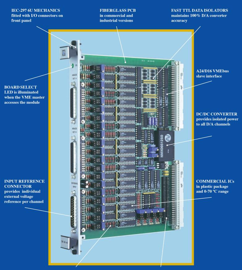
THIN FILM 0.1% RESISTORS improve converter accuracy
